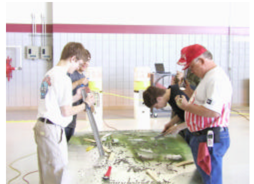
Cadets supervised by Bill Popejoy cleaning internal fuel tank parts of sealant.
